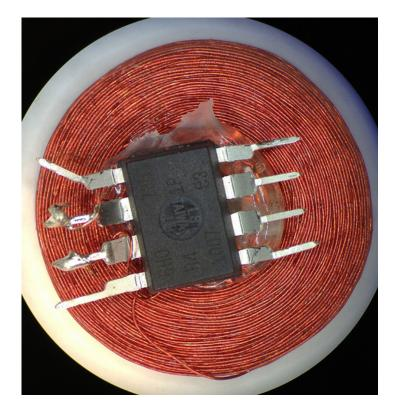
I was inspired by Beth's avrfid.S (http://scanlime.org/2010/06/avrfid-1-1-firmware/) project to try to build a replacement for the multiple HID Prox cards that I carry for work. Her design is simultaneously a technical tour-de-force and an example of how badly we can abuse the Atmel chips. Here is the entire schematic:
