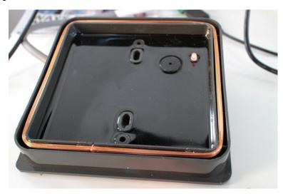
If you wanted to try to modify the firmware of the reader, you're out of luck. There are no user servicable parts inside -- the entirety of the body is filled with potting compound epoxy. If you're interested in lower level details and compatibility with multiple card formats, the proxmark3
