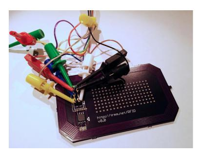
I've tried to make a PCB mount version that uses a long trace as the coil. It generates plenty of voltage, but for some reason that AVR isn't able to signal back to the reader. I tried to make the avr fit
