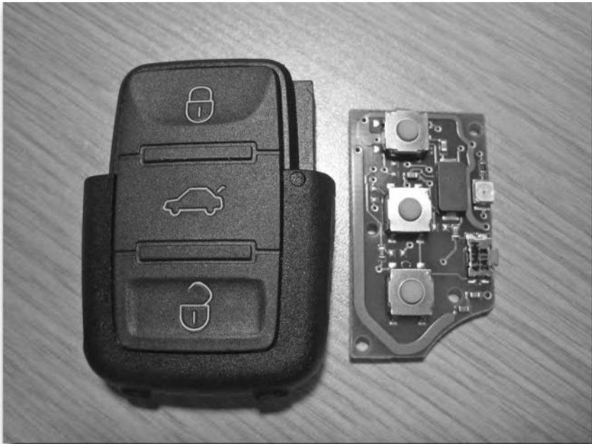
FIGURE 3-14: Casing with button faces and the button side of the remote board
